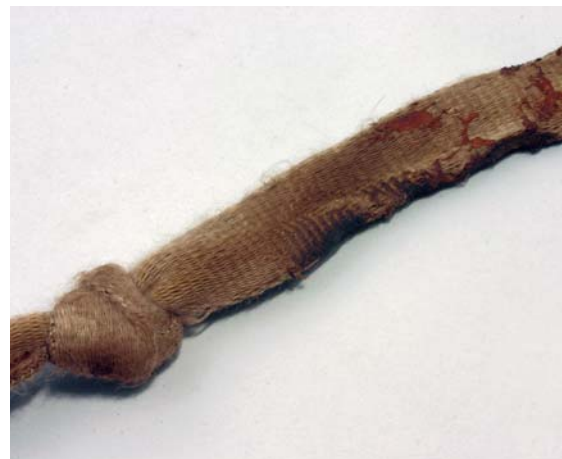
Knotted webbing with weld splatter.
