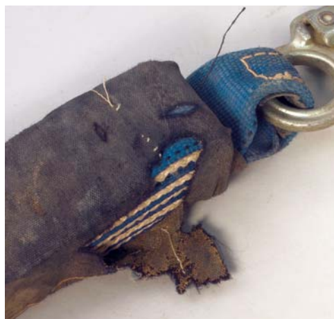
Damaged shock-absorber pack cover.
